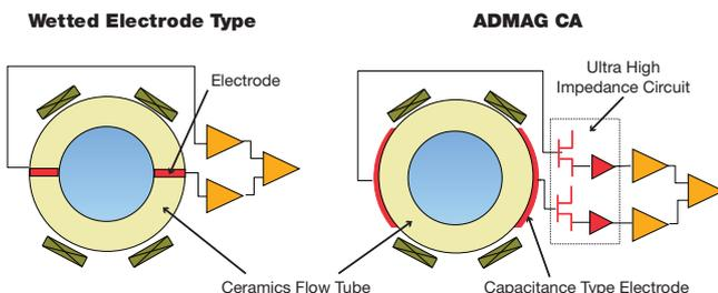
The benefits range from reducing slurry or process noise, eliminating potential leak paths and is for high coating process applications.
