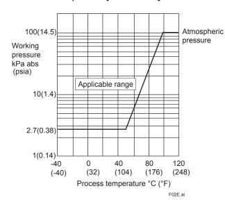
Figure 1-2. Working Pressure and Process Temperature [For EJA530E]
