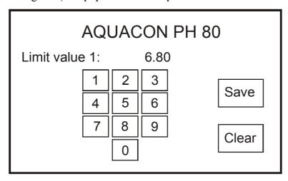
To leave the screen and confirm/safe the new parameter value, the button "Save" must be touched. To leave the screen without saving, the button "Clear" must be touched.
